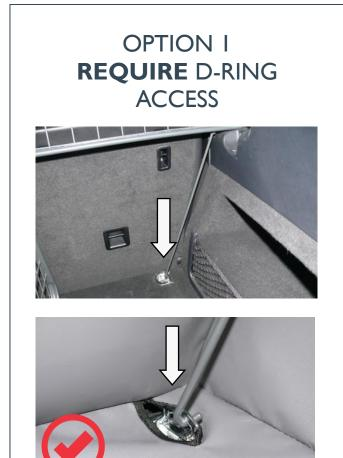
SLOT IN BOOT-LINER ALLOWS ACCESS TO D-RING
